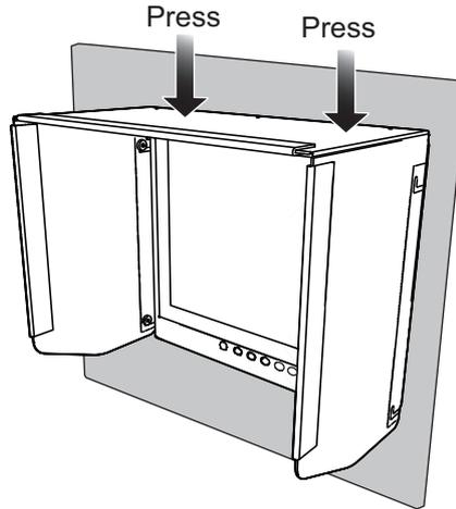
8. Fasten the knobs (4 places) to secure the hood (15) assembly in place.
