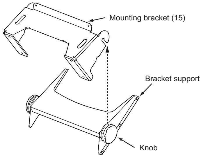
2. Secure the mounting bracket (15) to the mounting location with four self-tapping screws.
