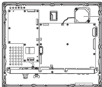
Fix the fan so that the label on the fan is directed downward, that is to the screen side.
