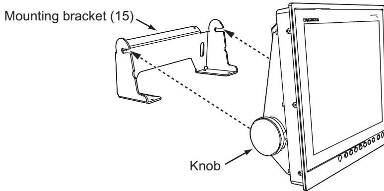
6. Adjust the angle of the monitor unit and fasten the knobs tightly.
