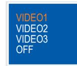
**Note 1:** To show the VIDEO1, VIDEO2 and VIDEO3 pictures alternately, set the cycle time (5 to 20 sec) with [PIP SW TIME] on the [OSD] menu. In this case, the above setting is invalid. See section 2.3.1.
