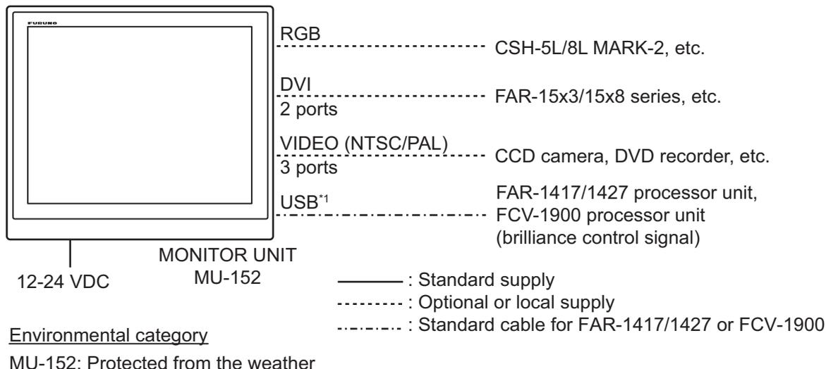
\*1: The USB port is for the brilliance control signal from the external equipment. You can not connect a PC or other device.
