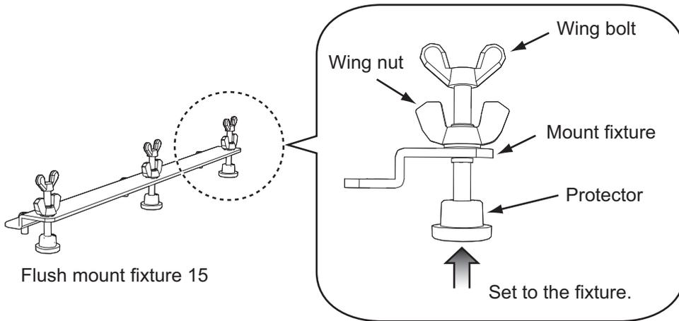
6. Fasten the flush mount fixture 15 to the right and left sides of the rear of the monitor unit with the washer head screws (6 places).
