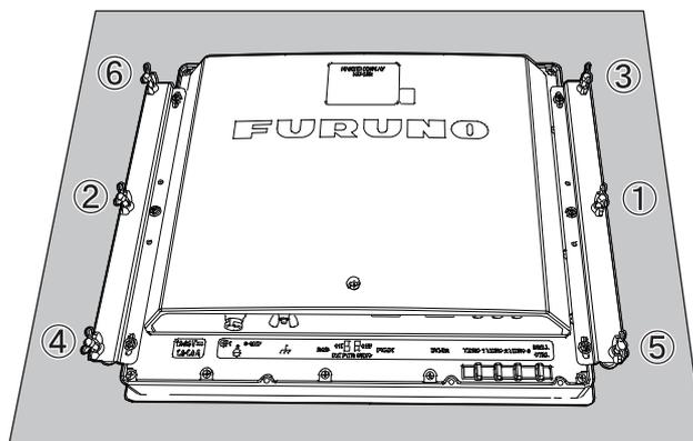
8. Fasten the wing bolts tightly, in the numerical order shown in step 7.
